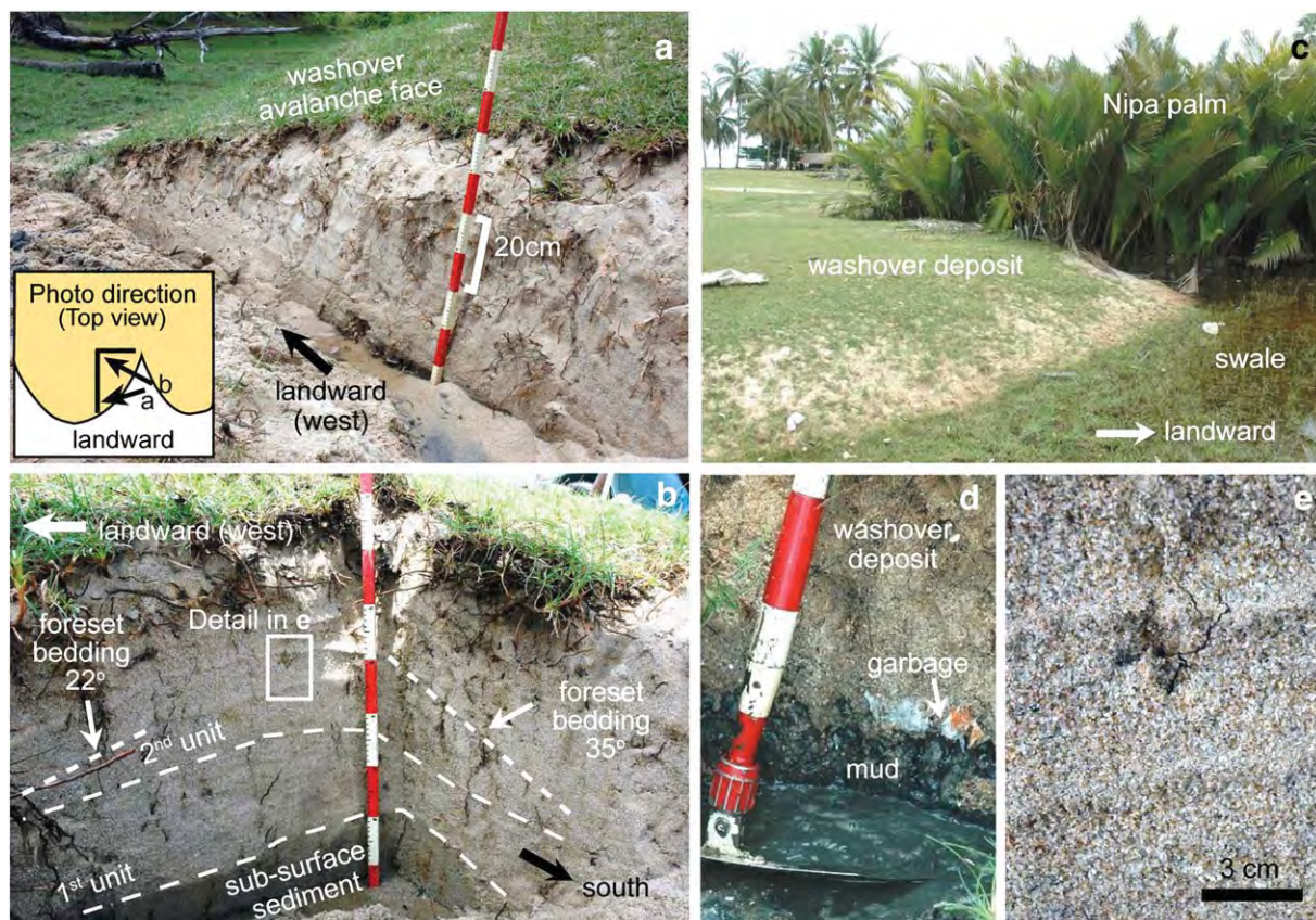
Fig. 5. (a) The washover successions and steeply avalanched face at the washover margin. (b) Two units within the washover deposit and foreset bedding at the distal end of the washover deposits. (c) Nipa palm in swale was partially buried by washover sediment. (d) Bottom sharp contact of washover sediment and mud in swale. (e) Reverse grading layer in the washover sediment.
