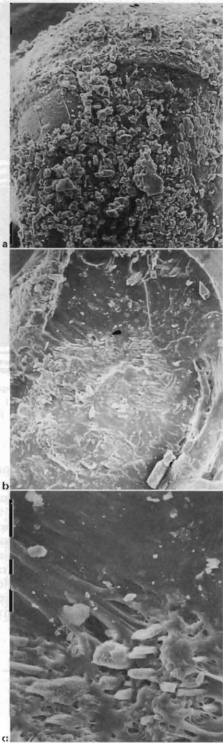
a capsule surface ( \times 30 ); b capsule cross-section ( \times 30 ); c capsule cross-section ( \times 150 )
