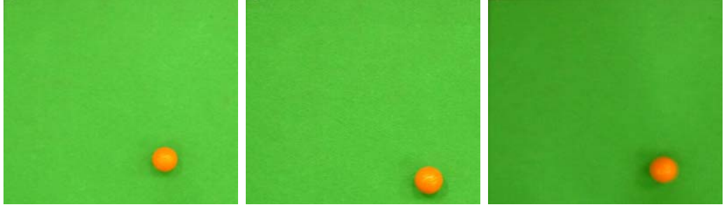
Figure 24: Real images of an orange golf ball on the green carpet. The three images were taken from three different illuminations (different light settings). From left to right: “Image1,” “Image2,” and “Image3.”
