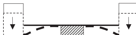
Fig. 3. Specimens loaded in bending.
