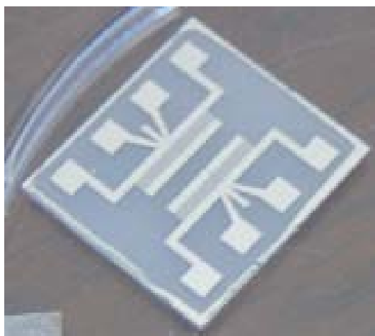
Fig. 1. A typical sensor showing two identical resonators.
