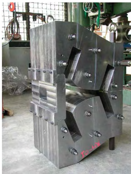
Fig. 7. (a) A pole piece lamination of the alpha magnet, (b) alpha-magnet poles, and (c) alpha-magnet assembly.
