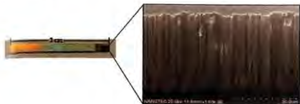
Fig. 2. Photograph of fabricated electrode and SEM micrograph of V-CNTs electrochemical electrode.
