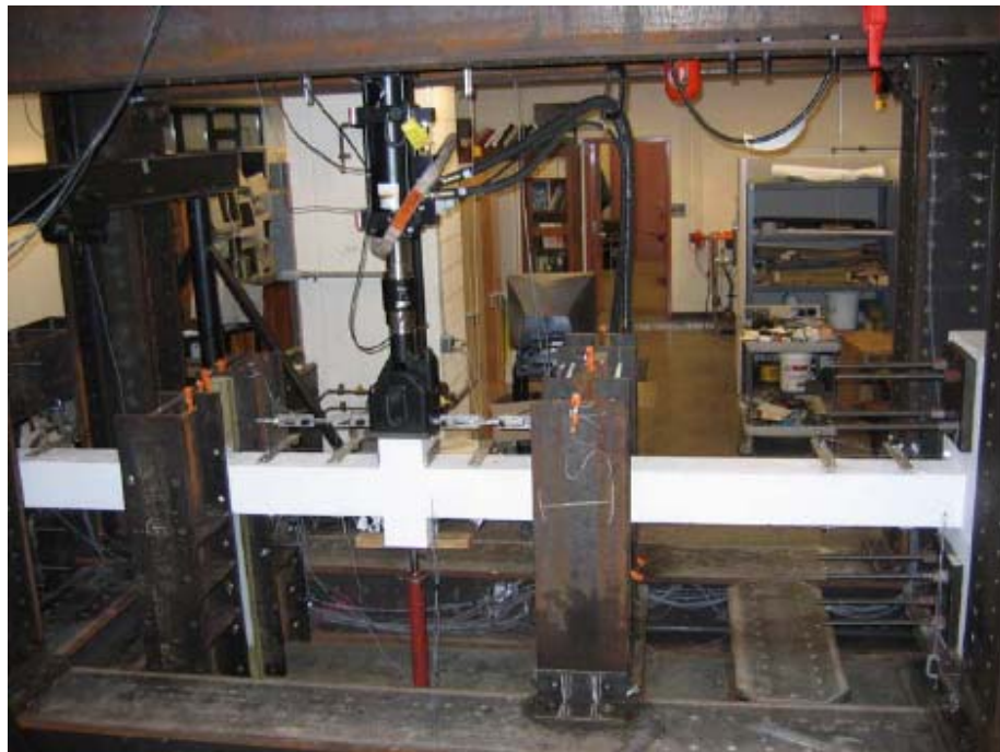
Figure 4-21 Bazan' s Two-Span Beam Specimen Installed on Steel Reaction Frame (Bazan, 2008)
