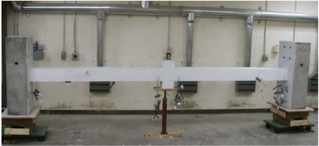
Figure 4-20 Bazan' s 3/8^{\text{th}} Scaled Two-Span Beam Specimen (Bazan, 2008)
