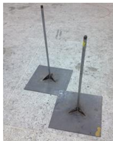
Fig. 5. Surface settlement plate
