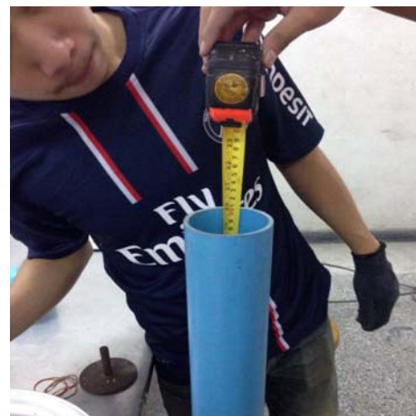
Figure 4.16 Fill the fine aggregate in the container to
