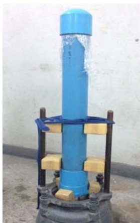
Figure 4.17 Seal the top of the container and vibrate for 24 minutes.
