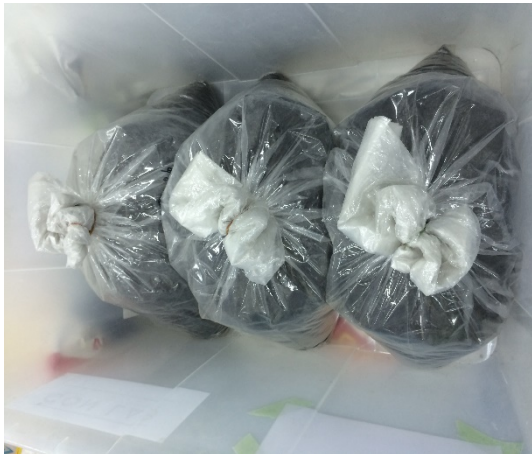
Figure 4.15 Keeping the fine aggregate for 24 hr.
