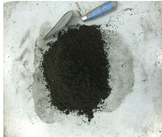
Figure 4.14 Mix the fine aggregate and water together.
