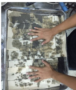
Figure 4.8 Wipe the aggregate by paper towel.
