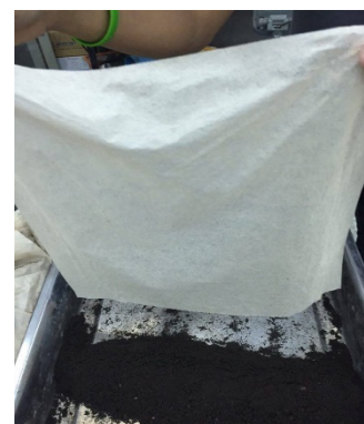
Figure 4.9 Wipe the aggregate until the surface- dry.
