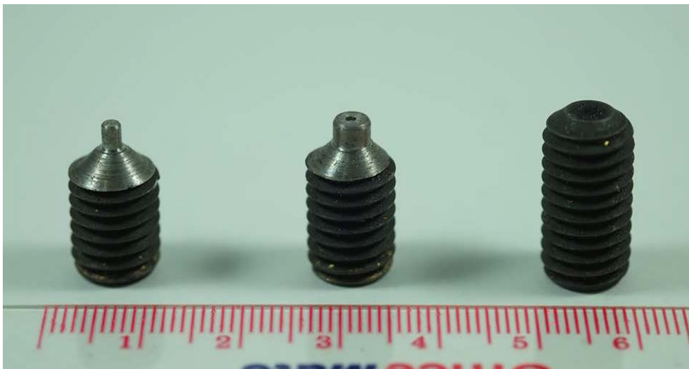
Figure 3.7 Three levels of screw contact area (3 mm 2 , 13 mm 2 and 24 mm 2 ) used in this study.
