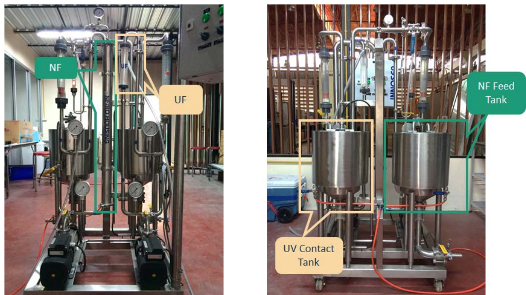
Figure 2.21 The hybrid NF membrane and photocatalysis operation unit
