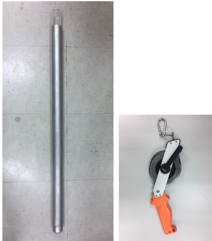
Figure 2.8 Bailer sampler for groundwater sampling
