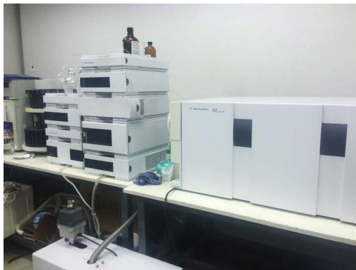
Figure 2.12 HPLC coupled with MS/MS
