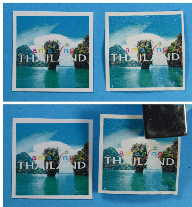
Fig. 10 (upper) Demonstration of the printability of the white magnetic paper (right), compared to the same image printed on standard A4 80 gsm paper (left). (lower) The printed white magnetic paper can be lifted by a magnet.
