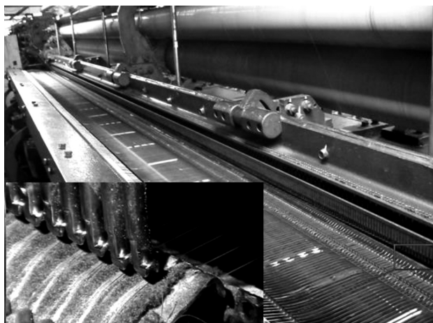
Figure 1: Fishing-net weaving machine and the upper hooks
