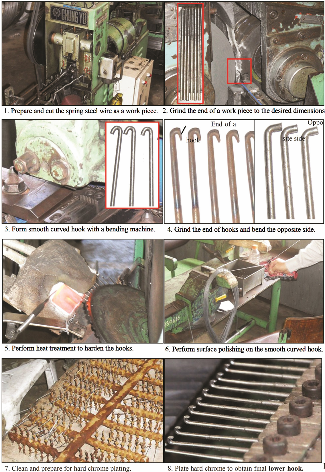
Fig. 1 – Lower hook manufacturing process
