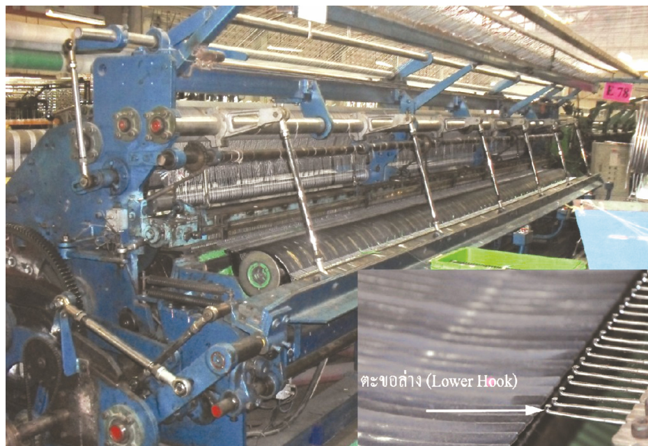
Fig. 2 – Fishing net-weaving machine and the lower hooks
