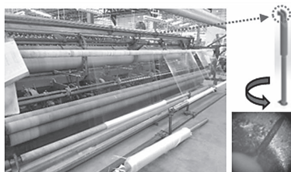
Figure 1 The damage to hooks on fishing net weaving process.
