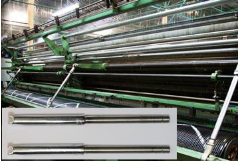
Fig. 1 A fishing net-weaving machine with inset of the upper hooks
