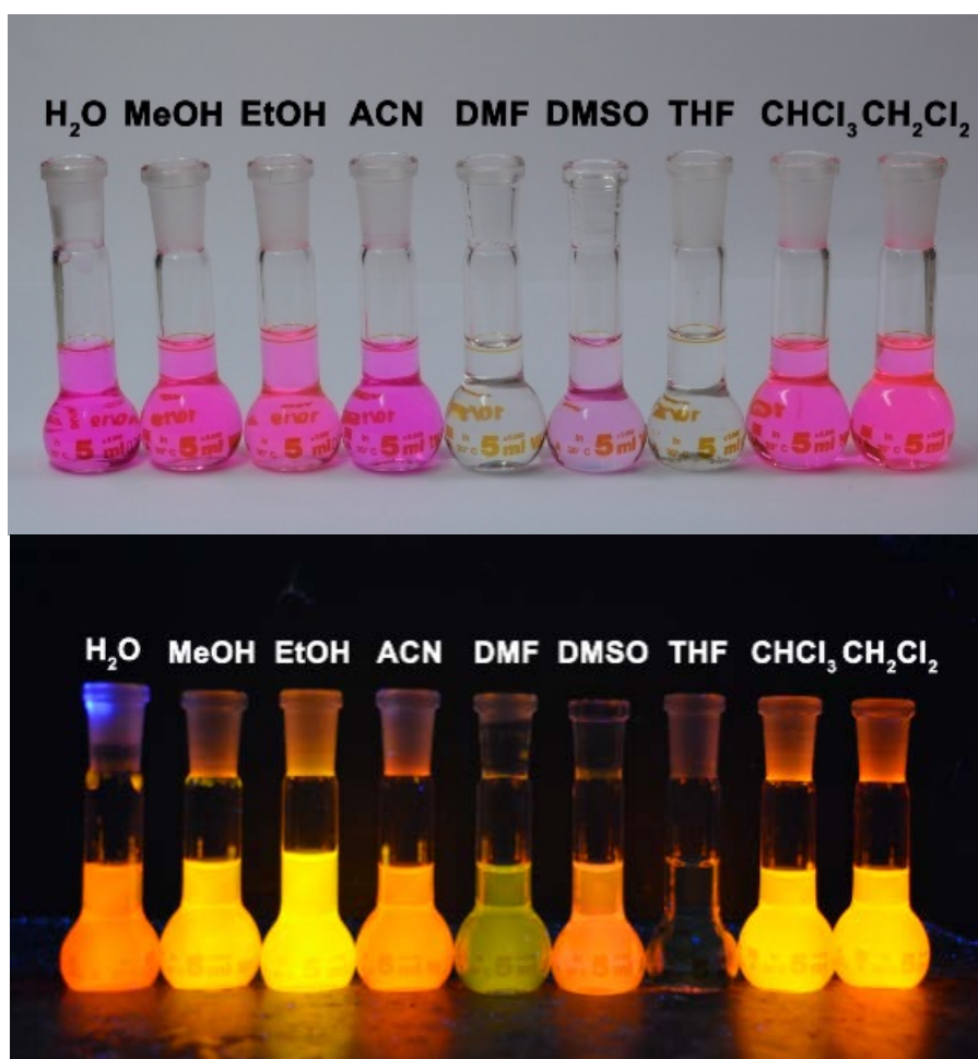
Fig. 2. Digital images of rhodamine B in different solvents at 10\ \mu\text{M} taken under normal illumination (above) and demonstrating skeletal fluorescence under 365nm illumination (below).
