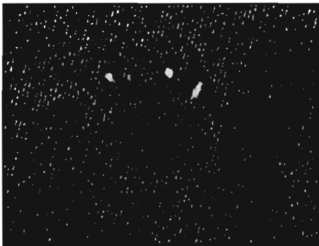
FIG. 6 Image of the four argon beam spots as seen on the beam profile monitor
