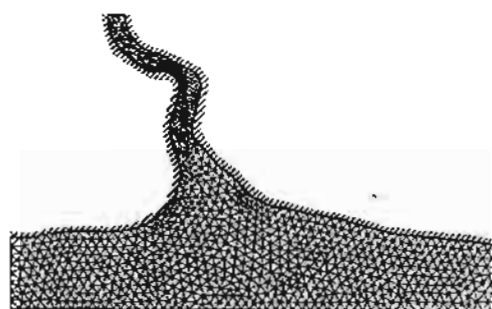
Fig. 13 Second finite element mesh for flow in Chao Phraya river
