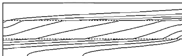
Fig. 7 Predicted temperature contours for the conjugate counter flow heat exchanger
