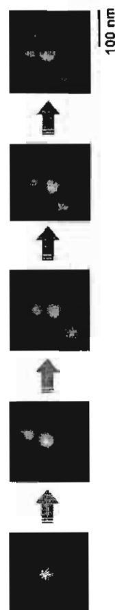
Fig. 3 AFM images showing the evolution of QDM with 4 satellite dots.
