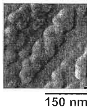
Figure 3 Aligned QDMs at 1.2 ML regrowth thickness
