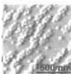
Fig. 3 QDMs are sets of QDs with specific pattern and with dot density of 10^{10} \text{ cm}^{-2}
