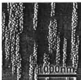
Fig. 2 AFM image of InAs QDMs grown by thin-capping-and-regrowth MBE process.
