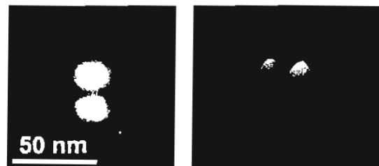
Fig. 5 Quantum dot pairs grown by gas-source MBE
