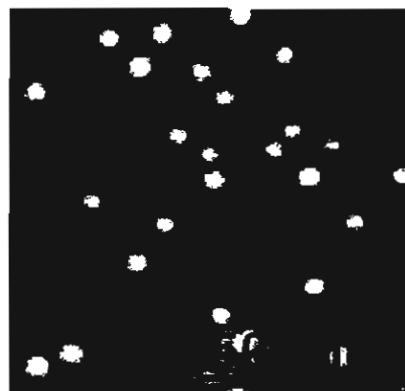
Fig. 1. AFM image of self-assembled InAs QDs on GaAs substrate.
