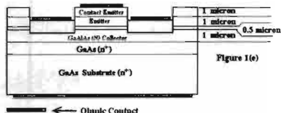
Figure 1. Schematic transistor sequence processes (a) LPE epitaxial layers. (b) Define the regrown base area. (c) Regrow the p + -GaAs base layer. (d) Define the intrinsic emitter-base area and uncover the contact emitter. (e) Ohmic contact formation
