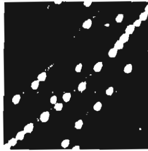
Fig. 5 Self-aligned quantum dots grown by repeating thin capping and regrowth three times.
