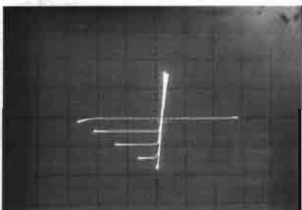
Figure 6. Inverted mode current-voltage characteristic of ST52, I_E : 1 mA/div, V_{CE} : 1 volt/div, I_B : 100 \mu A/step
