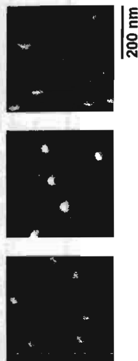
Fig. 1. AFM images of 0.6-ML InAs QDs regrown on nanohole templates previously formed at 470, 450 and 430°C, from left to right.
