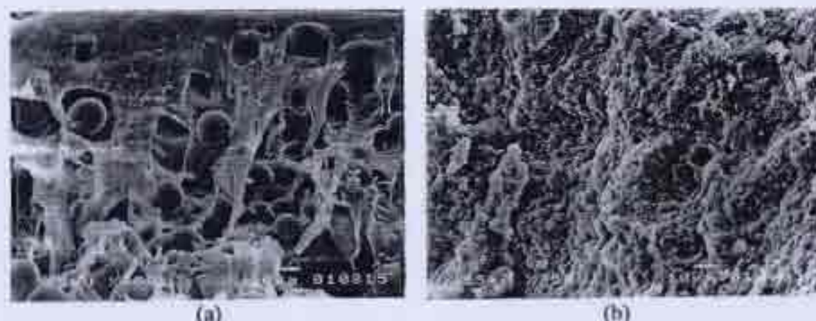
Figure 2. SEMs of cryogenic polymer fracture surface: (a) Polymer fracture of PP-block-EP (polymer 5); (b) polymer fracture of PP (polymer 6). ×750.
