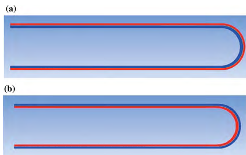
Fig. 5. Flow patterns in curved microchannel with surface modification of phase feed flow rates at (a) 0.025 mL/min with outer toluene and (b) 1 mL/min with outer water.
