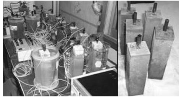
Fig. 2. Accelerated corrosion test with impressed voltage.
