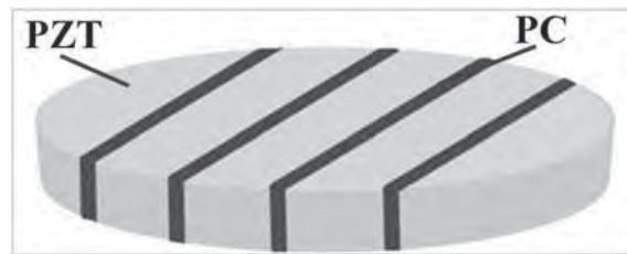
Figure 1. Schematic diagram of the 2–2 PZT-cement composite.
