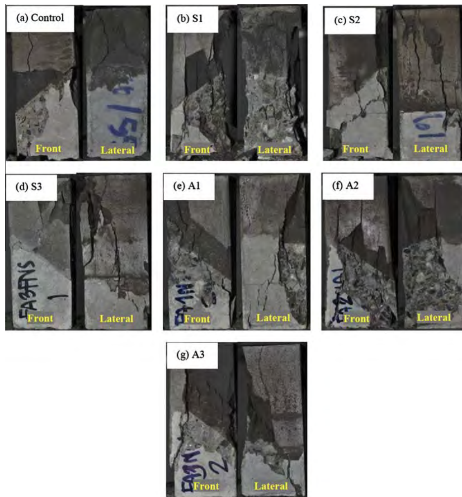
Fig. 10. Specimens failure mode at 28 days.
