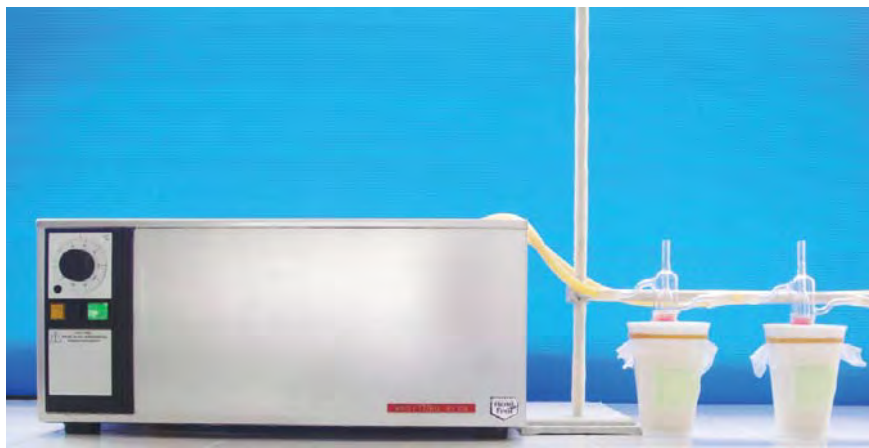
Figure 5. Artificial feeding system. A warm water-bath at 40°C, with a water pump placed inside, is connected to glass inlet and outlet feeding-chambers by rubber tubes. Thin paraffin-membrane covers the bottom tip of the feeding chambers, which are filled with human heparinized-blood, and the bottom tip is in close contact with 50 fasted adult female An. campestris -like Form E that are inside a screen-topped paper cup.
