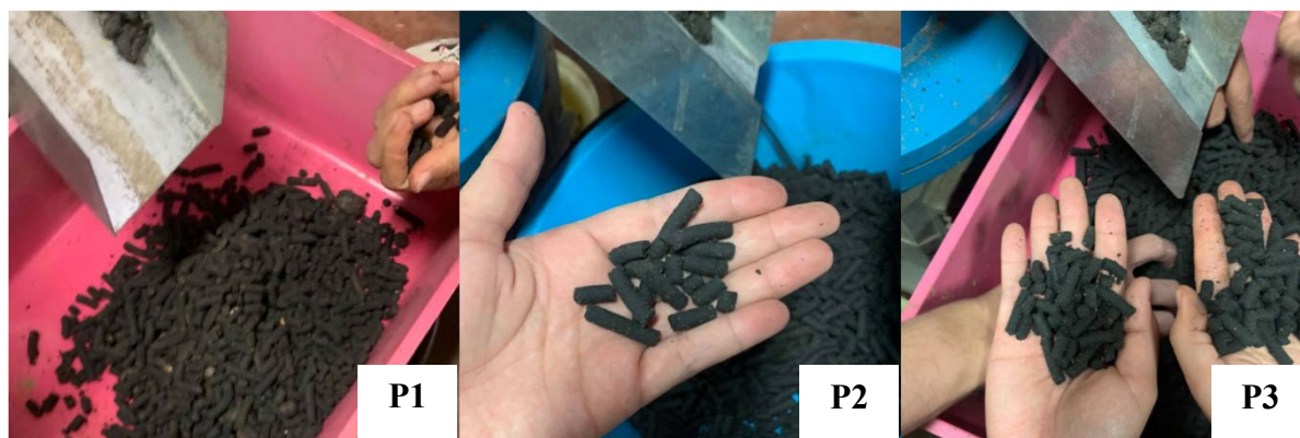
Figure 1. Pelleted bio-fertilizer formed by a fertilizer pellet machine at the Faculty of Engineering with different times of the pelleted process. P1 = the first time of pellet production, P2 = the second time of pellet production, P3 = the third time of pellet production.
