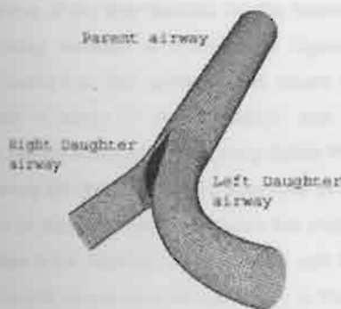
Figure 2 Three-dimensional mesh model of an asymmetric single bifurcation of the central airway
