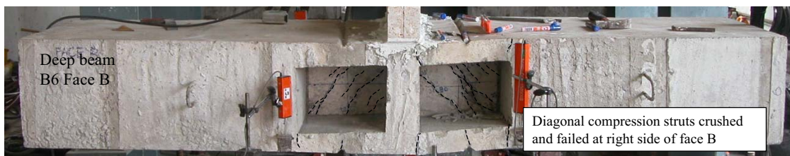
Shear capacity of control beam (Beam B6)
