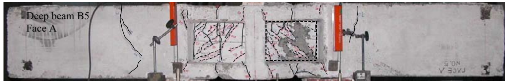
Shear capacity of deep beam B5
