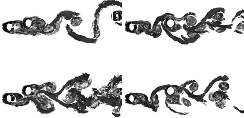
Figure 2: Instantaneous vorticity surfaces. Top to bottom: T/D=0.5 , T/D=1.0 and Left to Right: L/D=2.5 , L/D=5.0 , dark gray and light gray are stream-wise vorticity and span-wise vorticity, respectively
