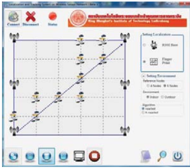
Figure 12. Result of Moving Target for 6 Reference Nodes in GUI using fingerprint-based technique
