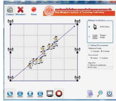
Figure 9. Result of Moving Target for 6 Reference Nodes in GUI using range-based technique
