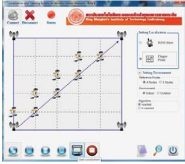
Figure 11. Result of Moving Target for 4 Reference Nodes in GUI using fingerprint-based technique
