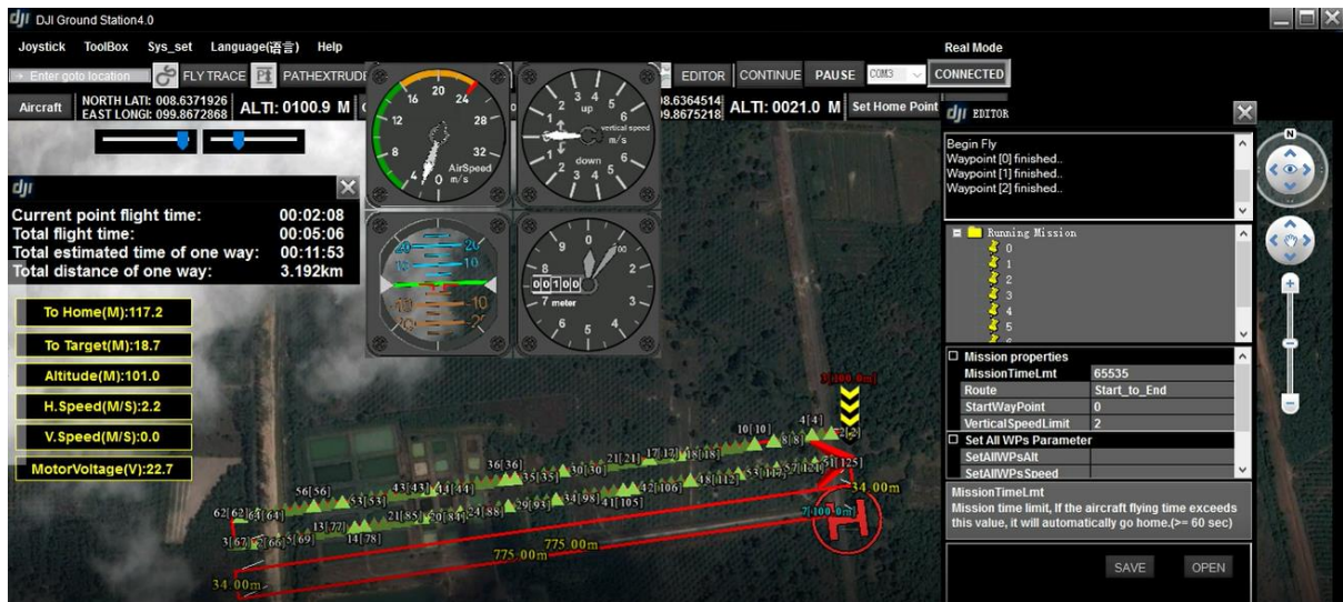
Figure 5.11: PC ground station control UAV autopilot for taking pictures along each flight plan
