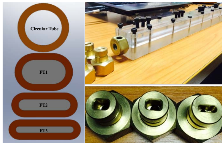
Fig. 3.3 The cross section of tested tube and the photograph of the test section and test section header
