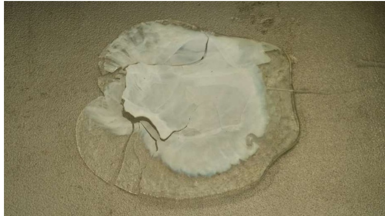
Figure 6 Partially crystallised glass sample in tin borate system (SnB15)
