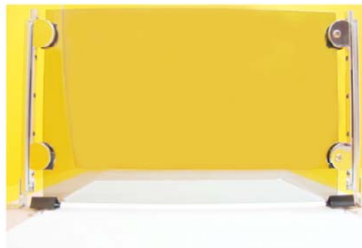
Figure 2. Setting the small gap, 2 mm height, between the semi-transparent glass and the graph paper using two paper clips, which permits the drawing of a ray diagram.
