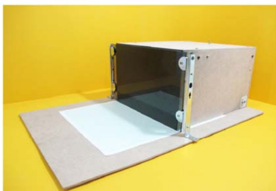
Figure 3. The black box is used to cover the other half of the wooden plate to demonstrate that an image formed by the semi-transparent glass and a plane mirror is the same. A thin iron metal plate is fixed under the wooden plate using nuts and bolts to attract magnets inside the cube.
