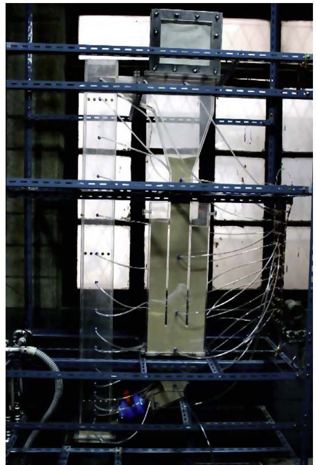
Fig. 1. The configuration of the experimental CFBR used in this study.
