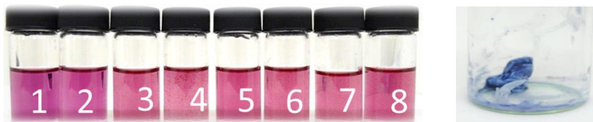
Fig 5 Variation of number of EBT droplets (1-8 drops) containing 50 \text{ mg.L}^{-1} \text{ Mg}^{2+} in DI water a) and precipitation of NRL sample when 3 drops of EBT were applied b) .
