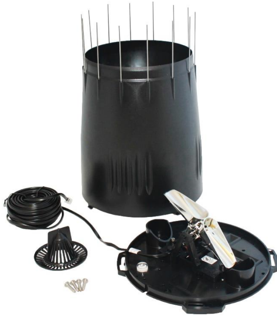
Fig. 32. The Davis Instruments Rain Collector 7852.
