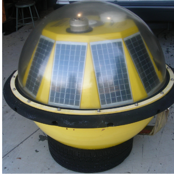
Figure 4.17: Triaxy's solar-powered and telemetry-equipped wave buoy.
