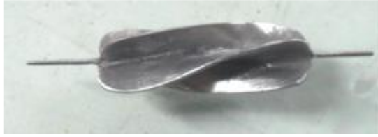
a) Turbine type swirl generator inserts (Duangthongsuk & Wongwises [10, 11])
